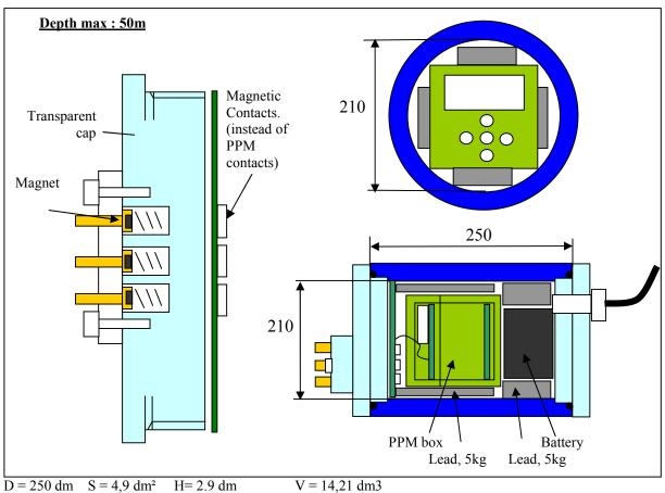
$\overline{D} = 250 \text{ dm}$  S = 4,9 dm<sup>2</sup> H= 2.9 dm V = 14,2 Battery 7AH 0.7 x 0.9 x 1.5 = 0.95 dm3
